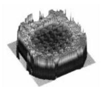
A surface plot from MIT's Full-Wafer Imaging Interferometer, showing full-wafer etching rate uniformity.
