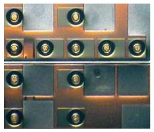
Figure 11. Technology for inductive/capacitive chip-to-package connection
